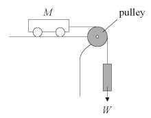
The cart is connected to an object of weight W via a pulley. Which of the following is the acceleration of the cart?
