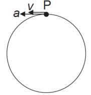
A mass connected to one end of a rigid rod rotates at constant speed in a vertical plane about the other end of the rod.
