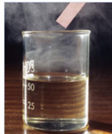
Figure 3.1.12 Silicon(IV) chloride, \text{SiCl}_4 , even reacts with water vapour in the air, producing an acidic vapour that turns blue litmus paper pink.
