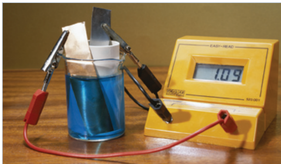
Figure 8.0.1 A Daniell cell is made up of a copper electrode (often a copper container) with a porous partition separating the copper sulfate solution from the zinc sulfate solution. A zinc anode is in the centre of the cell.
