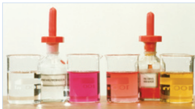
Figure 7.6.1 The acid–base indicator phenolphthalein is colourless in acidic solutions and a pink-purple colour in alkaline solutions, whereas methyl orange is red in acidic solutions and yellow in alkaline solutions.
