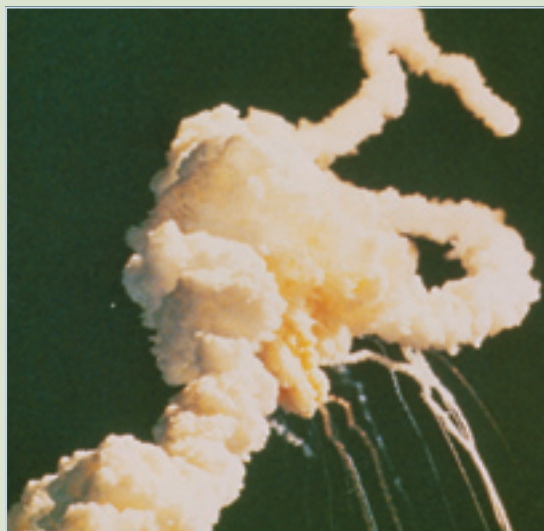
Figure 5.2.6 The Challenger disaster—the result of a hydrogen–oxygen explosion. A faulty o-ring allowed the hydrogen and oxygen to mix, resulting in a chain reaction explosion.
