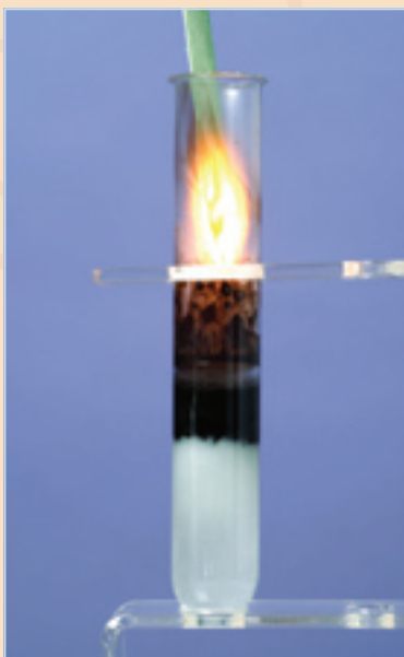
Figure 3.2.11 The decomposition of hydrogen peroxide can be catalysed by the black powder, MnO 2 . The rate at which oxygen is released is dramatically increased and easily re-lights a glowing splint.
