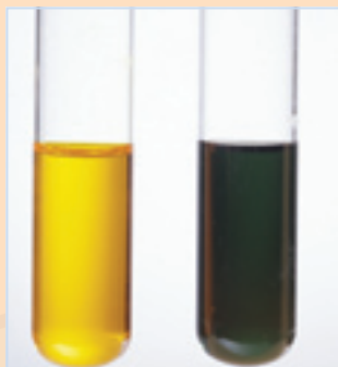
Figure 3.2.4 When ethanol is oxidized by potassium dichromate, the orange \text{Cr}_2\text{O}_7^{2-} ion is reduced to the dark green \text{Cr}^{3+} ion.
