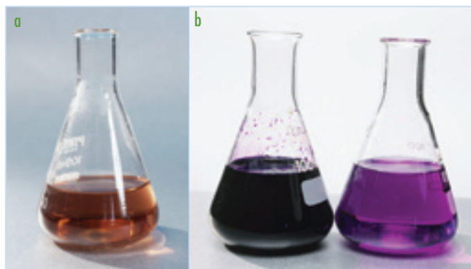
Figure 3.2.3 Manganese can be found in a range of oxidation states including (a) manganese(III) and (b) manganese(VII).
