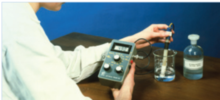
Figure 7.2.1 The pH of a dilute solution of ethanoic acid can be determined experimentally using a pH meter.
