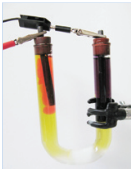
Figure 8.2.8 When water is reduced, hydroxide ions increase the pH of the solution (on right) and when it is oxidized, hydrogen ions decrease the pH of the solution (on left).
