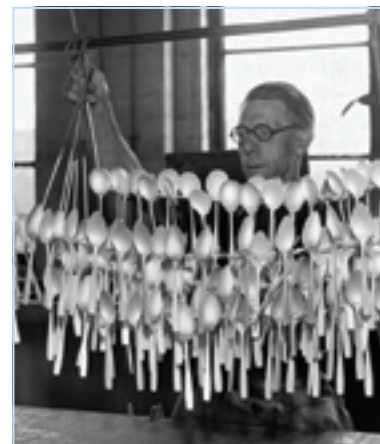
Figure 8.2.12 Spoons to be electroplated are prepared for an electrolyte bath.
