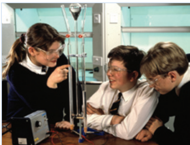
Figure 8.2.6 A voltmeter is used to electrolyse aqueous solutions and to collect the gases produced.
