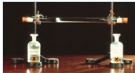
Figure 4.4.2 The formation of ammonium chloride is clearly demonstrated when cotton wool balls soaked in HCl and \text{NH}_3 are placed at either end of a tube and the vapours diffuse towards each other.
