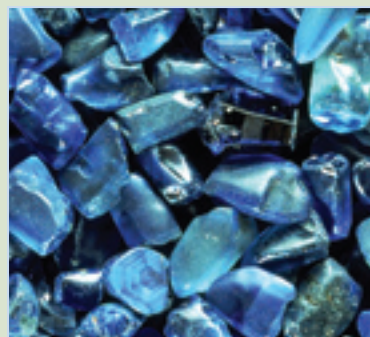
Figure 3.1.5 Sapphire is a form of corundum, \text{Al}_2\text{O}_3 . These sapphires were separated from river gravel by panning.
