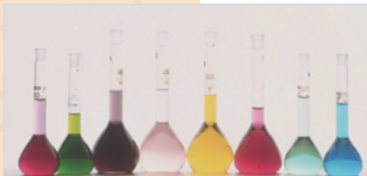
Figure 3.3.8 Transition metal compounds exhibit a wide range of colours. From left to right the solutions are compounds of titanium (Ti), vanadium (V), chromium (Cr), manganese (Mn), iron (Fe), cobalt (Co), nickel (Ni) and copper (Cu).
