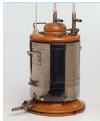
Figure 4.1.2 The standard enthalpy change of combustion could be measured in a bomb calorimeter.
