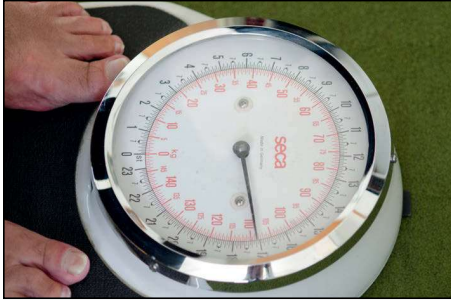
Figure 2.40 The familiar bathroom scales do not measure mass. They measure the force that you exert on the scales. This force is equal to the weight only when the scales are at rest.
