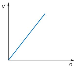
To increase the charge on the capacitor by a small change of charge  $\delta q$  requires work  $\delta q V$  to be done. This is represented by the area of the thin strip in the graph.
