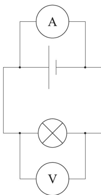
25. A lamp is connected to an electric cell and it lights at its working voltage. The lamp is then connected to the same [1 mark] cell in a circuit with an ideal ammeter and an ideal voltmeter. Which circuit allows the lamp to light at the original brightness?
