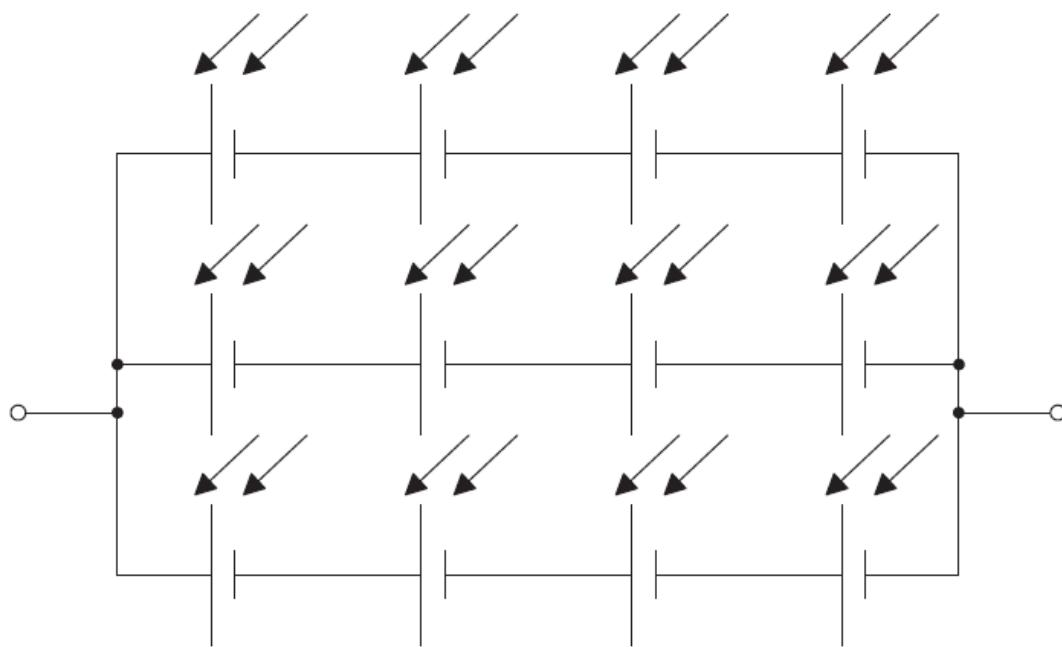
Each cell in the module has an emf of  $0.75\text{V}$  and an internal resistance of  $1.8\Omega$ .
