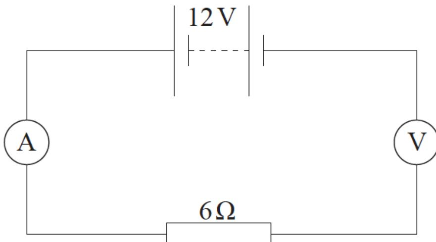
What is the reading on the ammeter and on the voltmeter?
