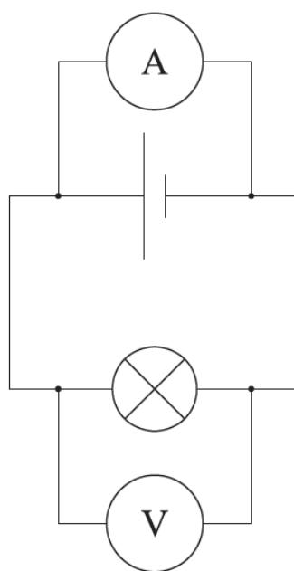
26. A voltmeter of resistance  $50\text{k}\Omega$  is used to measure the electric potential difference in a circuit, as shown. The cell [1 mark] has an electromotive force (emf) of 5.0V and negligible internal resistance.
