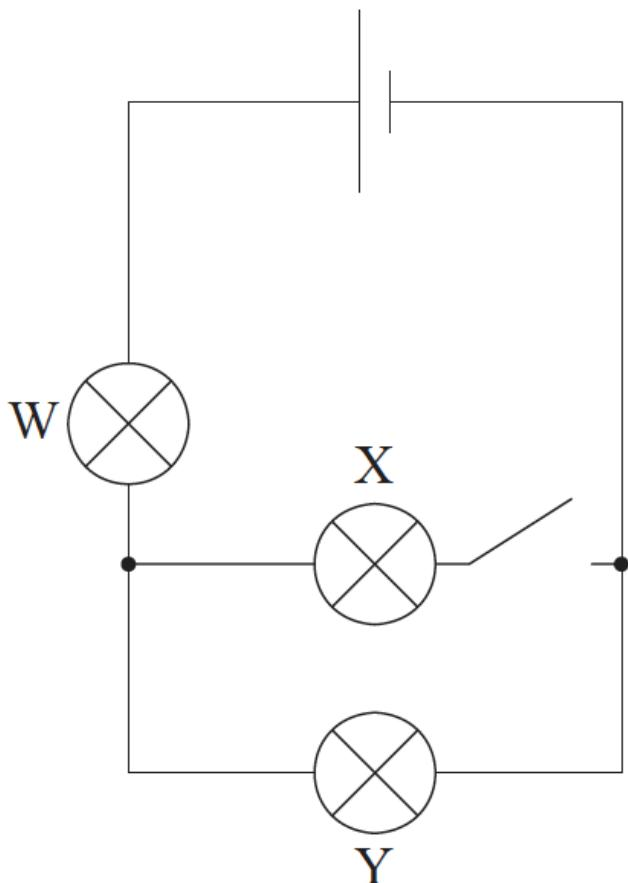
When the switch is closed, all the lamps light. Which of the following correctly describes what happens to the brightness of lamp W and lamp Y when the switch is opened?
