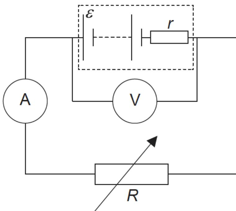
The variable resistor  $R$  is adjusted and the values of potential difference  $V$  across the cell and current  $I$  are recorded. Which graph shows the variation of  $V$  with  $I$ ?
