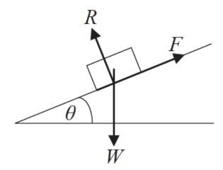
The normal reaction acting between the block and the plane is R and the frictional force between the block and the plane is F. The incline is at an angle  $\theta$  to the horizontal. What is the magnitude of F?
