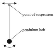
For each value of the driving frequency a steady constant amplitude A is reached. The oscillations of the pendulum bob are lightly damped.
