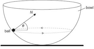
The normal reaction force N makes an angle  $\theta$  to the horizontal.
