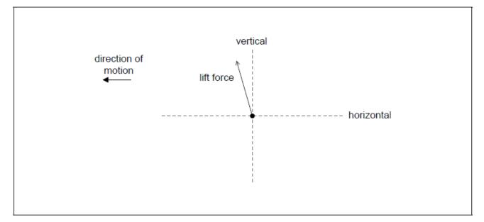
Draw the forces acting on the glider to complete the free-body diagram. The dotted lines show the horizontal and vertical directions.
