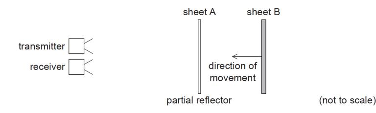
Sheet A is fixed and sheet B is moved towards it. While sheet B is moving, the intensity of the signal detected at the receiver goes through a series of maximum and minimum values.
