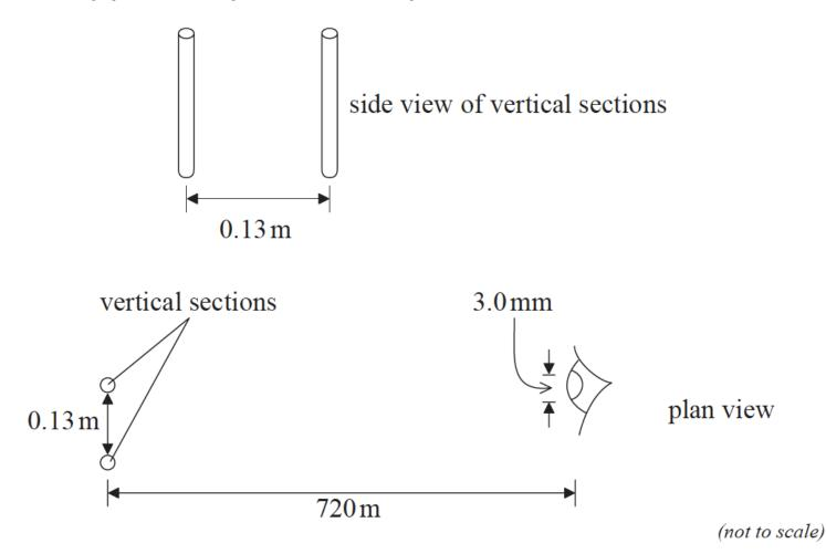
The vertical sections are separated by a horizontal distance of 0.13 m. An observer views them from a distance of 720 m. The wavelength of the emitted light is 510 nm and the diameter of the aperture of the observer's eye is 3.0 mm.
