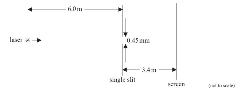
After passing through the slit, the light is incident on a screen that is a distance of 3.4 m from the slit. Calculate the distance between the centre and the first minimum of the diffraction pattern.
