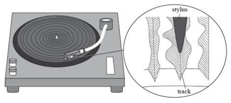
As the LP record rotates, the stylus moves because of changes in the width and position of the track. These movements are converted into sound waves by an electrical system and a loudspeaker.
