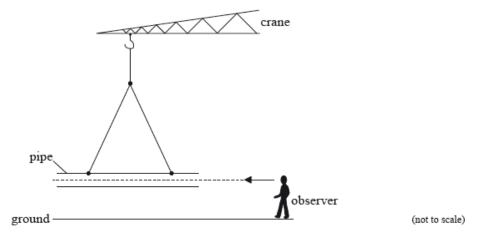
Wind blows across one end of the pipe. This causes a standing wave to form in the air of the pipe, producing the first harmonic. The pipe has a length of 2.1 m and the speed of sound in air is  $330 \text{ m s}^{-1}$ .
