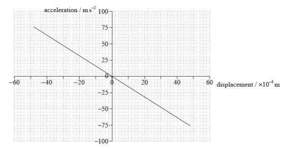
The mass of the stylus is  $5.5 \times 10^{-4}$  kg. Determine the maximum kinetic energy of the stylus.
