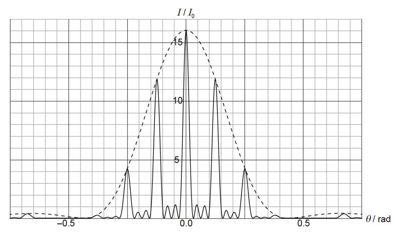
$I_0$  is the intensity of the light at the middle of the screen from **one** slit.
