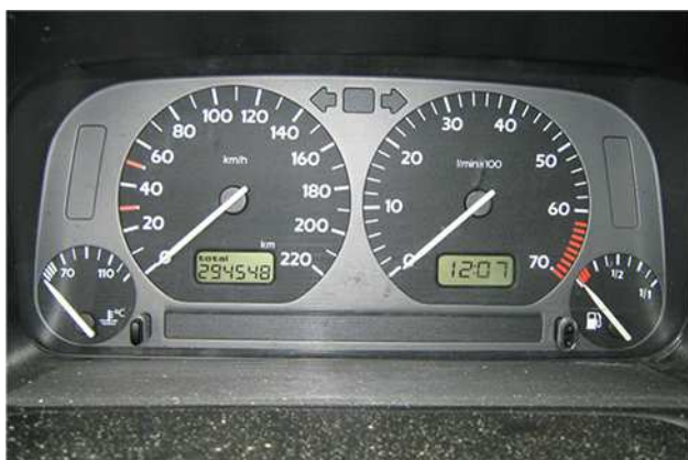
Figure 10.34 The fuel and temperature gauges (far right and far left, respectively) in this 1996 Volkswagen are voltmeters that register the voltage output of “sender” units. These units are proportional to the amount of gasoline in the tank and to the engine temperature. (credit: Christian Giersing)
