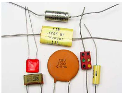
Figure 8.4 These are some typical capacitors used in electronic devices. A capacitor's size is not necessarily related to its capacitance value. (credit: Windell Oskay)
