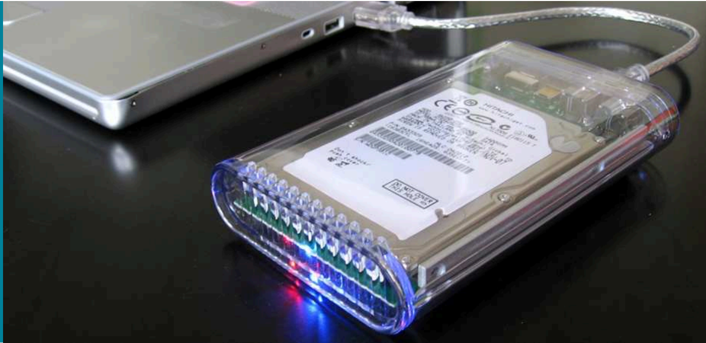
Figure 12.1 An external hard drive attached to a computer works by magnetically encoding information that can be stored or retrieved quickly. A key idea in the development of digital devices is the ability to produce and use magnetic fields in this way. (credit: modification of work by “Miss Karen”/Flickr)
