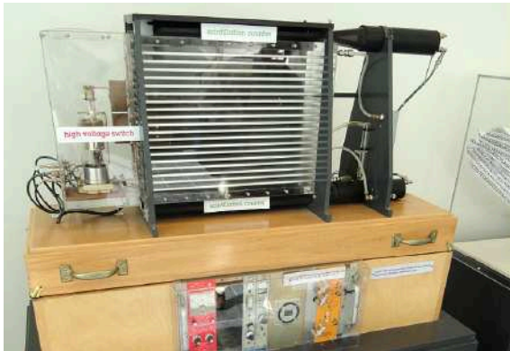
Figure 7.16 A spark chamber is used to trace the paths of high-energy particles. Ionization created by the particles as they pass through the gas between the plates allows a spark to jump. The sparks are perpendicular to the plates, following electric field lines between them. The potential difference between adjacent plates is not high enough to cause sparks without the ionization produced by particles from accelerator experiments (or cosmic rays). This form of detector is now archaic and no longer in use except for demonstration purposes. (credit b: modification of work by Jack Collins)
