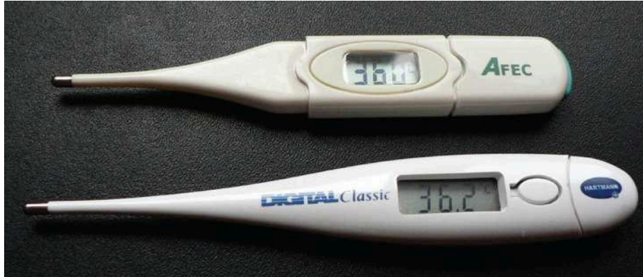
Figure 9.17 These familiar thermometers are based on the automated measurement of a thermistor's temperature-dependent resistance.
