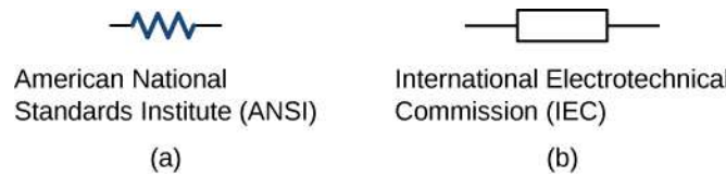
Figure 9.14 Symbols for a resistor used in circuit diagrams. (a) The ANSI symbol; (b) the IEC symbol.
