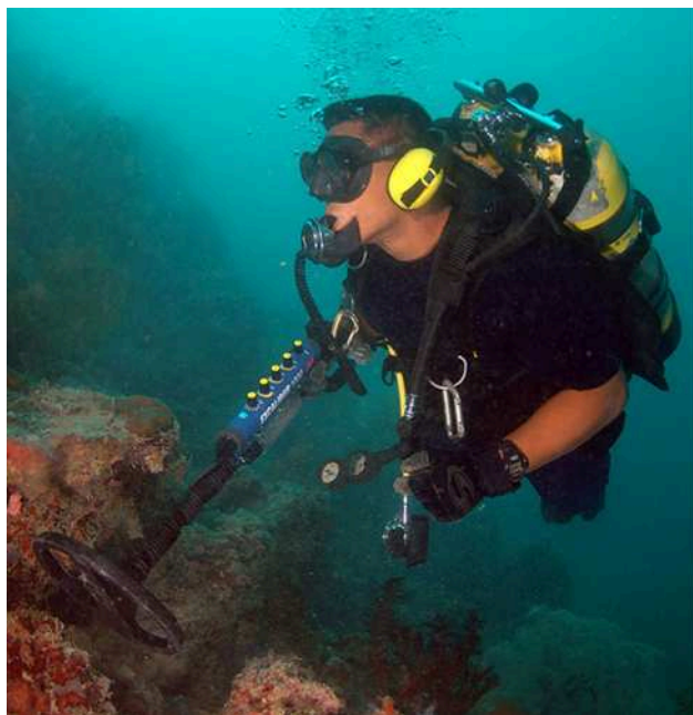
Figure 15.19 When a metal detector comes near a piece of metal, the self-inductance of one of its coils changes. This causes a shift in the resonant frequency of a circuit containing the coil. That shift is detected by the circuitry and transmitted to the diver by means of the headphones. (credit: modification of work by Eric Lippmann, U.S. Navy)
