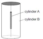
At the start of the experiment all the air was removed from cylinder B. The alpha particles combined with electrons as they moved through the wall of cylinder A to form helium gas in cylinder B.
