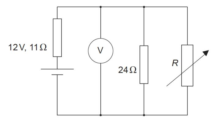
Power supplies deliver maximum power to an external circuit when the resistance of the external circuit equals the internal resistance of the power supply.
