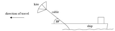
The tension in the cable that connects the kite to the ship is 250 kN. The kite is pulling the ship at an angle of  $39^{\circ}$  to the horizontal. The ship travels at a steady speed of  $8.5 \text{ m s}^{-1}$  when the ship's engines operate with a power output of 2.7 MW.
