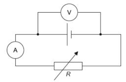
The variable resistor is adjusted and a series of current and voltage readings are taken. The graph shows the variation with *R* of the power dissipated in the cell and the power dissipated in the variable resistor.
