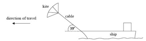
The tension in the cable that connects the kite to the ship is 250 kN. The kite is pulling the ship at an angle of 39° to the horizontal. The ship travels at a steady speed of  $8.5 \text{ m s}^{-1}$  when the ship's engines operate with a power output of 2.7 MW.
