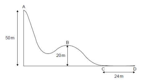
A skier of mass 65 kg starts from rest at point A and during the ski course some of the gravitational potential energy transferred to kinetic energy.
