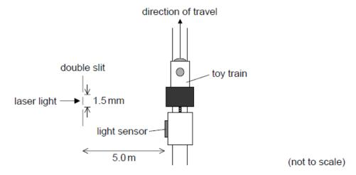
Light from a laser is incident on a double slit. The light from the slits is detected by a light sensor attached to the train.
