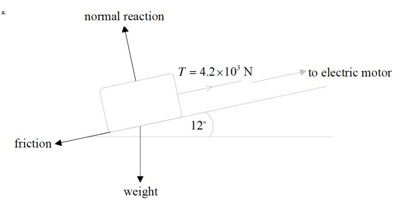
(normal) reaction/N/R and weight/force of gravity/gravity force/gravitational force/mg/w/W with correct directions; friction/frictional force/*F*/*F*<sub>f</sub> with arrow pointing down ramp along surface of ramp; Do not allow "gravity" as label. Do not allow "drag" as label for friction.
