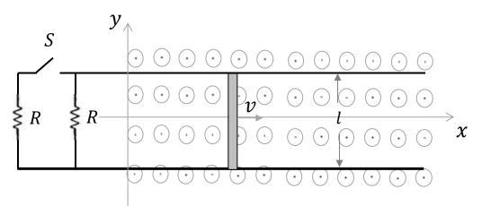
a. Since the velocity is constant, an external force  $F_H$  must act on the rod. Determine the magnitude and direction of this force.
