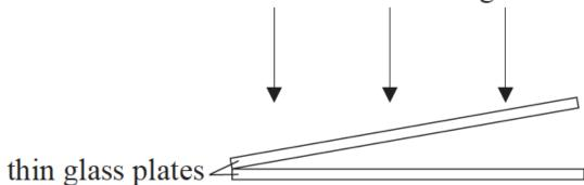
A beam of monochromatic light is incident on the air wedge. The reflected light is observed through a microscope and a pattern of equally spaced parallel fringes is observed.
