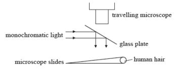
A hair is used to separate two microscope slides. A monochromatic beam of light is reflected onto the two slides by the glass plate. The light is then reflected from the two slides and transmitted through the glass plate and is viewed by the travelling microscope.
