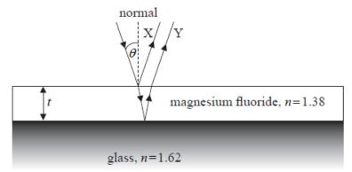
X is a ray reflected from the surface of the film and Y is reflected from the surface of the glass.
