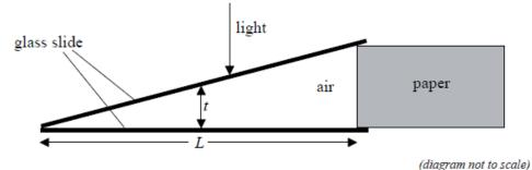
A thin wedge of air of variable thickness, *t*, is trapped between the two slides. The arrangement is viewed normally from above, using light of wavelength 590 nm. The glass plates are coated, so that reflection only takes place at the bottom surface of the top plate and the top surface of the bottom plate.
