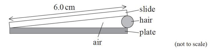
An observer viewing the microscope slide at near-normal incidence measures the fringe spacing to be 0.29 mm. Calculate the thickness of the hair.
