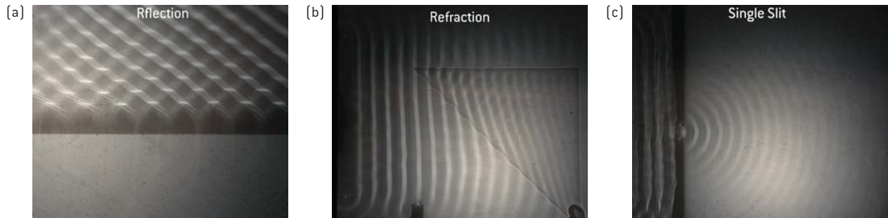
▲ Figure 2 Reflection, refraction, and diffraction of waves in a ripple tank.
