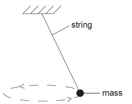
A mass is suspended by a string from a fixed point. The mass moves with constant speed along a circular path in a horizontal plane.
