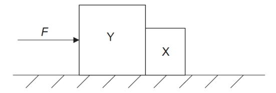
The blocks remain in contact as they accelerate along a horizontal frictionless surface. Y has a greater mass than X. Air resistance is negligible.
