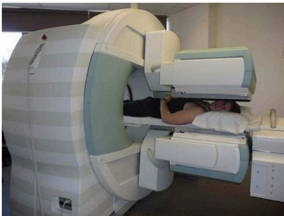
Figure 10.28 The SPECT machine uses radiopharmaceutical compounds to produce an image of the human body. The machine takes advantage of the physics of nuclear beta decays and electron-positron collisions. (credit: "Woldo"/Wikimedia Commons)
