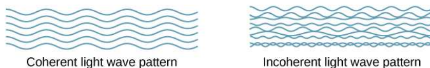
Figure 8.29 A coherent light wave pattern contains light waves of the same frequency and phase. An incoherent light wave pattern contains light waves of different frequencies and phases.
