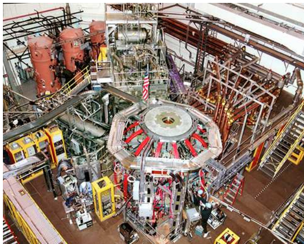
Figure 5.25 The National Spherical Torus Experiment (NSTX) is a fusion reactor in which hydrogen isotopes undergo fusion to produce helium. In this process, a relatively small mass of fuel is converted into a large amount of energy. (credit: Princeton Plasma Physics Laboratory)
