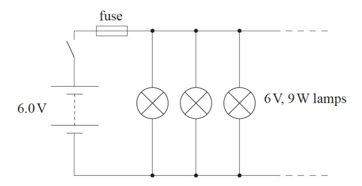
The diagram shows three 6V, 9W lamps connected in parallel to a supply of emf 6.0V and negligible internal resistance. A fuse in the circuit melts if the current in the circuit exceeds 13A.
