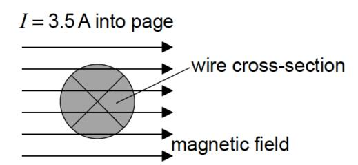
The wire which carries a current of 3.5A into the page, is placed in a region of uniform magnetic field of flux density 0.25T. The field is directed at right angles to the wire.
