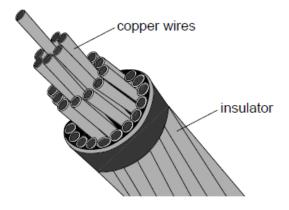
The cable consists of 32 copper wires each of length 35 km. Each wire has a resistance of 64  $\Omega$ . The resistivity of copper is 1.7 x 10<sup>-8</sup>  $\Omega$  m.
