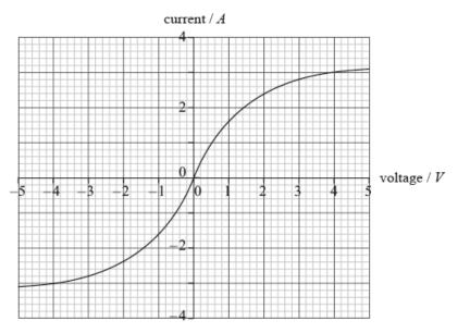
Component X is now connected across the terminals of a cell of emf 2.0 V and negligible internal resistance. Use the graph to show that the resistance of X is  $0.83 \Omega$ .
