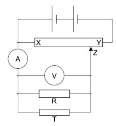
Slider Z of the potentiometer is moved from Y to X.
