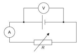
The variable resistor is adjusted and a series of current and voltage readings are taken. The graph shows the variation with *R* of the power dissipated in the cell and the power dissipated in the variable resistor.
