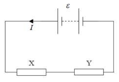
The power dissipated in each of the two resistors is the same.
