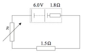
Estimate the resistance R of the variable resistor that will limit the current to 0.82A.
