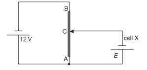
AB is a wire of uniform cross-section and length 1.0 m. The resistance of wire AB is 80  $\Omega$ . When the length of AC is 0.35 m the current in cell X is zero.
