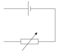
The variable resistor is set to  $1.5 \Omega$ . When the cell converts 7.2 mJ of energy, 5.8 mC of charge moves completely around the circuit. The potential difference across the variable resistor is 0.55 V.
