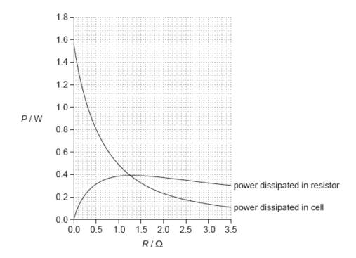
The cell has an internal resistance.
