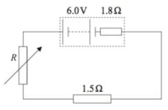
Estimate the resistance R of the variable resistor that will limit the current to 0.82A.
