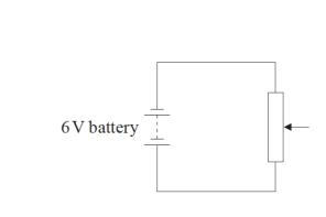
Draw the complete circuit showing the correct position of the bulb, ammeter and voltmeter.
