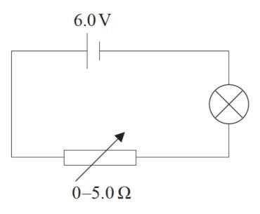
Explain, with a calculation, why this circuit will not allow for a full range of potential difference from 0 V to 6 V across the bulb. Assume that the resistance of the lamp remains constant at a value of  $2.4 \Omega$ .
