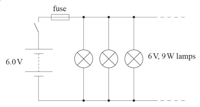
The diagram shows three 6V, 9W lamps connected in parallel to a supply of emf 6.0V and negligible internal resistance. A fuse in the circuit melts if the current in the circuit exceeds 13A.
