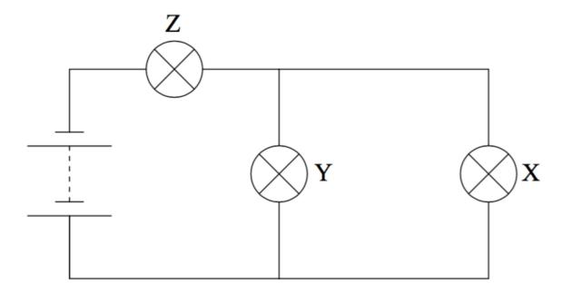
The filament of lamp X breaks. Which of the following correctly describes the change in brightness of lamp Y and of lamp Z?
