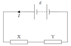
The power dissipated in each of the two resistors is the same.
