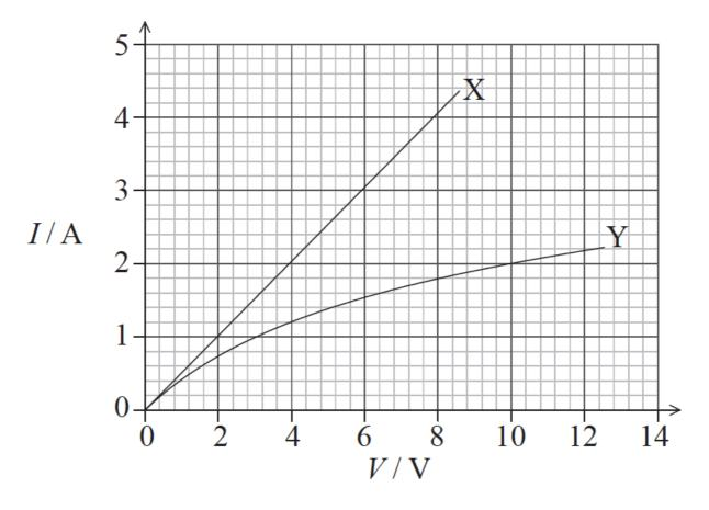
When resistors X and Y are connected in series, the current in the resistors is 2.0 A. What is the resistance of the series combination of X and Y?
