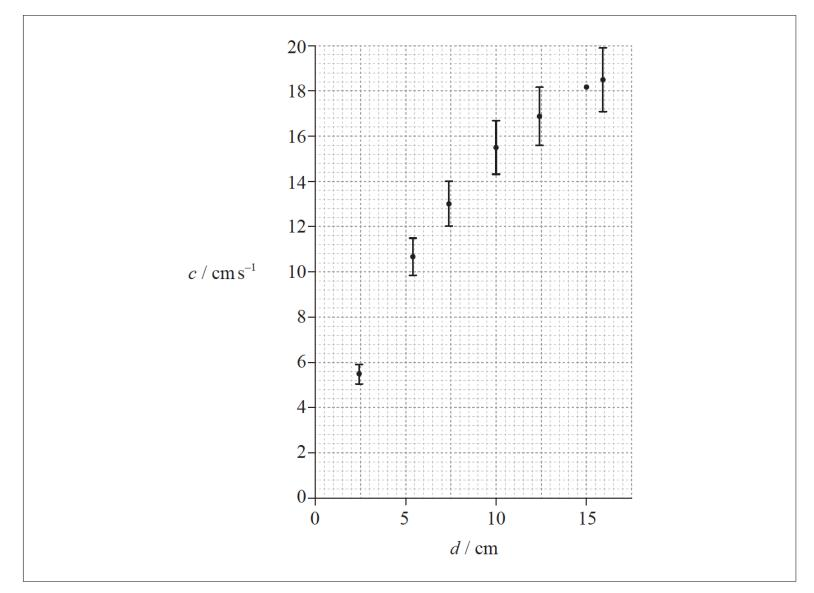
Caroline carried out an experiment to measure the variation with water depth *d* of the wave speed *c* of a surface water wave. Her data are shown plotted below.
