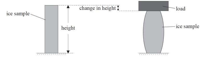
After the load has been applied, it is observed to move downwards at a constant speed v as the ice deforms. The constant speed v is measured for different loads. The graph shows the variation of v with load W for a number of identical samples of ice.
