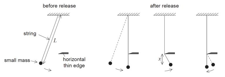
The length L of the string is kept constant during the experiment. The vertical position of the horizontal thin edge is varied to change x.
