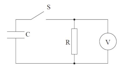
The initial potential difference across C was 12V. The switch S was closed and the potential difference *V* across R was measured at various times *t*. The data collected, along with error bars, are shown plotted below.
