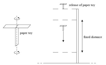
The aim of the experiment was to find how the terminal speed of the paper toy varies with its weight. The weight of the paper toy was changed by using different numbers of paper sheets in its construction.
