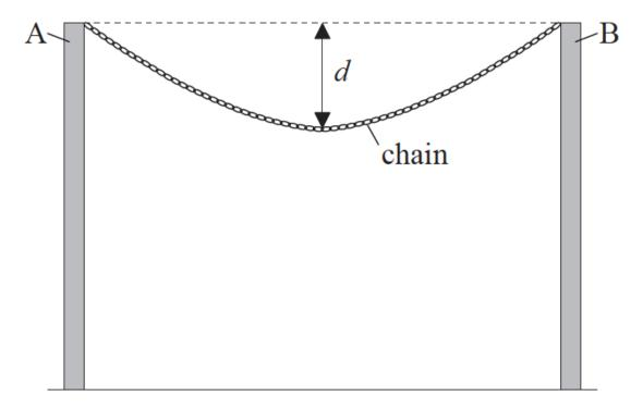
The length / of the chain can be increased by adding extra links. An experiment was undertaken to investigate how the sag *d* of the midpoint of the chain, measured from the horizontal between A and B, varies with *l*. The data obtained are shown plotted below. The uncertainties in *l* are too small to be shown.
