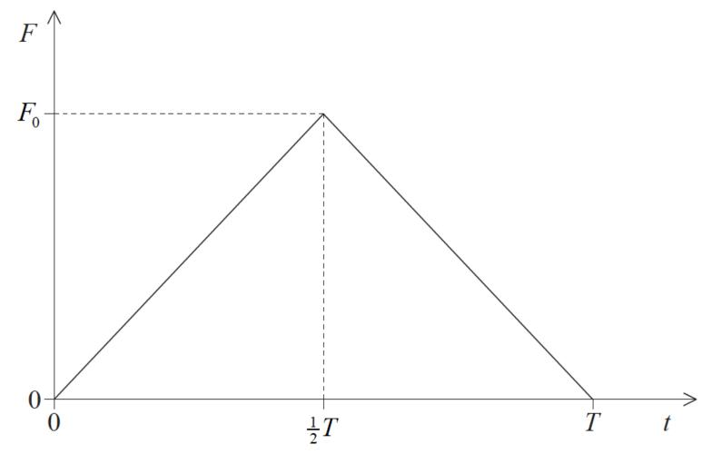
The maximum value of F is  $F_0$  and the total time of contact between ball and wall is T.
