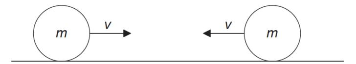
The spheres undergo a head-on elastic collision.
