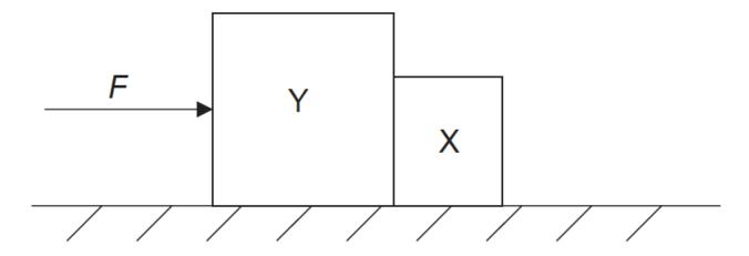
The blocks remain in contact as they accelerate along a horizontal frictionless surface. Y has a greater mass than X. Air resistance is negligible.
