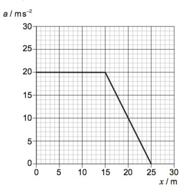
The mass of the object is 3.0 kg. What is the total work done on the object?
