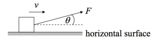
The block is moving with a constant velocity v along the surface. A resistive force acts on the block.
