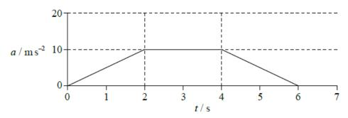
What is the magnitude of the change in the velocity of the object between 0 and 3 seconds?
