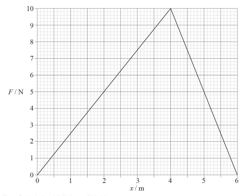
After travelling 6 m, the change in the kinetic energy of the body is
