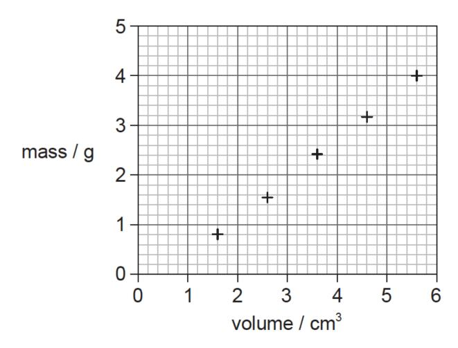
Using the information on the graph, what can be said about the measurements used to find the density of oil?
