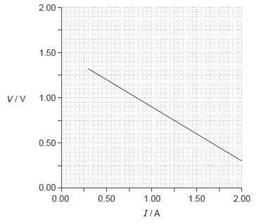
Using the graph, determine the best estimate of the internal resistance of the cell.
