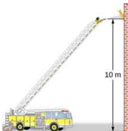
Figure 14.33 Pressure in the nozzle of this fire hose is less than at ground level for two reasons: The water has to go uphill to get to the nozzle, and speed increases in the nozzle. In spite of its lowered pressure, the water can exert a large force on anything it strikes by virtue of its kinetic energy. Pressure in the water stream becomes equal to atmospheric pressure once it emerges into the air.
