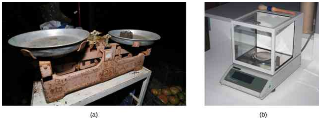
Figure 1.11 (a) A double-pan mechanical balance is used to compare different masses. Usually an object with unknown mass is placed in one pan and objects of known mass are placed in the other pan. When the bar that connects the two pans is horizontal, then the masses in both pans are equal. The “known masses” are typically metal cylinders of standard mass such as 1 g, 10 g, and 100 g. (b) Many mechanical balances, such as double-pan balances, have been replaced by digital scales, which can typically measure the mass of an object more precisely. A mechanical balance may read only the mass of an object to the nearest tenth of a gram, but many digital scales can measure the mass of an object up to the nearest thousandth of a gram. (credit a: modification of work by Serge Melki; credit b: modification of work by Karel Jakubec)
