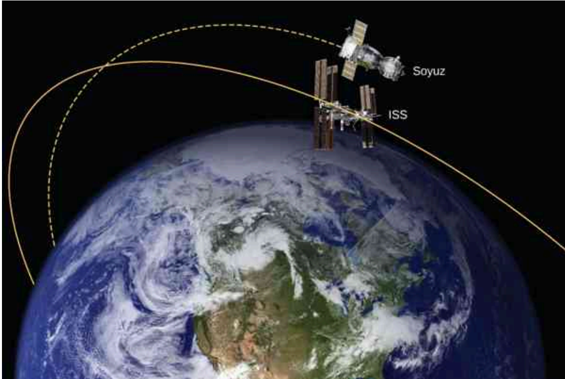
Figure 13.15 The Soyuz in a rendezvous with the ISS. Note that this diagram is not to scale; the Soyuz is very small compared to the ISS and its orbit is much closer to Earth. (credit: modification of works by NASA)
