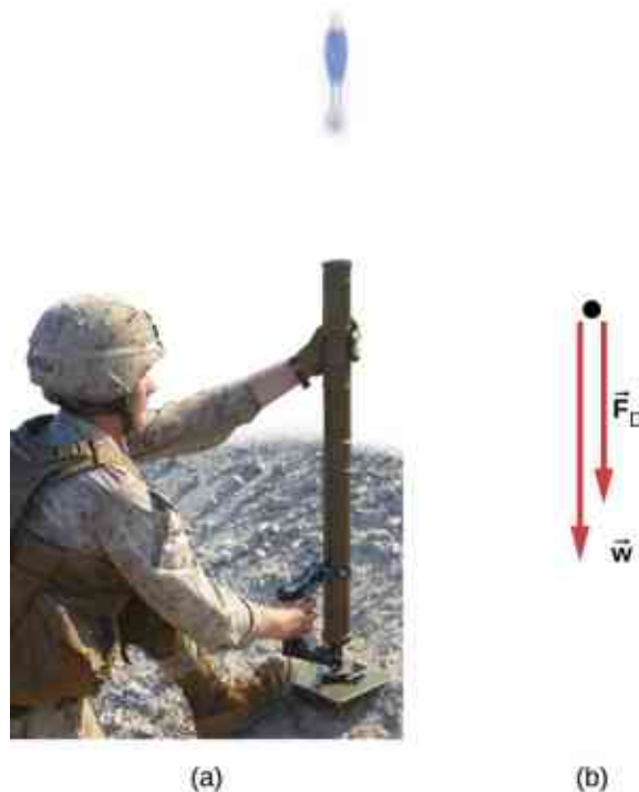
Figure 6.9 (a) The mortar fires a shell straight up; we consider the friction force provided by the air. (b) A free-body diagram is shown which indicates all the forces on the mortar shell. (credit a: modification of work by OS541/DoD; The appearance of U.S. Department of Defense (DoD) visual information does not imply or constitute DoD endorsement.)
