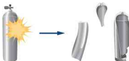
Figure 9.25 A scuba tank explodes into three pieces.
