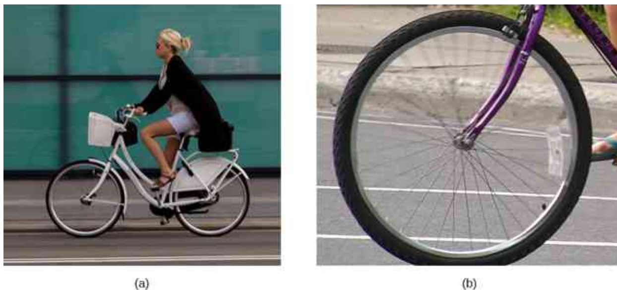
Figure 11.2 (a) The bicycle moves forward, and its tires do not slip. The bottom of the slightly deformed tire is at rest with respect to the road surface for a measurable amount of time. (b) This image shows that the top of a rolling wheel appears blurred by its motion, but the bottom of the wheel is instantaneously at rest. (credit a: modification of work by Nelson Lourenço; credit b: modification of work by Colin Rose)
