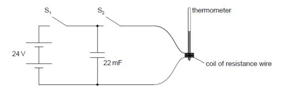
A power supply of emf (electromotive force) 24 V and of negligible internal resistance is connected to a capacitor and to a coil of resistance wire using an arrangement of two switches. Switch  $S_1$  is closed and, a few seconds later, opened. Then switch  $S_2$  is closed.
