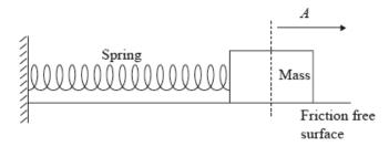
An identical mass is attached to an identical spring. The maximum displacement is 2A. Assuming this spring obeys Hooke's law, which of the following gives the correct time period and total energy?
