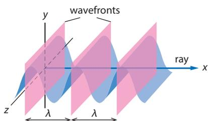
**b** A ray is the direction normal to wavefronts that corresponds to the direction of energy transfer.
