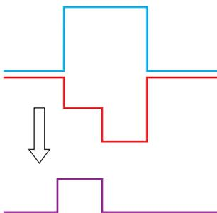
17 Adding the pulses point by point gives the following diagram.
