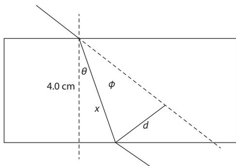
$1.00 \times \sin 40^\circ = 1.450 \times \sin \theta$ , hence  $\theta = 26.3^\circ$ . This means that  $x = \frac{4.0}{\cos 26.3^\circ} = 4.46$  cm.
