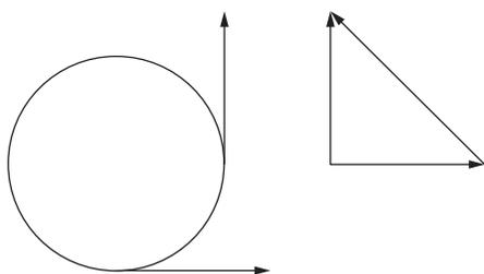
The magnitude of the velocity vector is  $4.0 \text{ m s}^{-1}$  and it takes a time of  $\frac{2\pi \times 2.0}{4.0} = 3.14 \text{ s}$  to complete a full revolution. Hence a time of  $\frac{3.14}{4} = 0.785 \text{ s}$  to complete a quarter of revolution from A to B. The magnitude of
